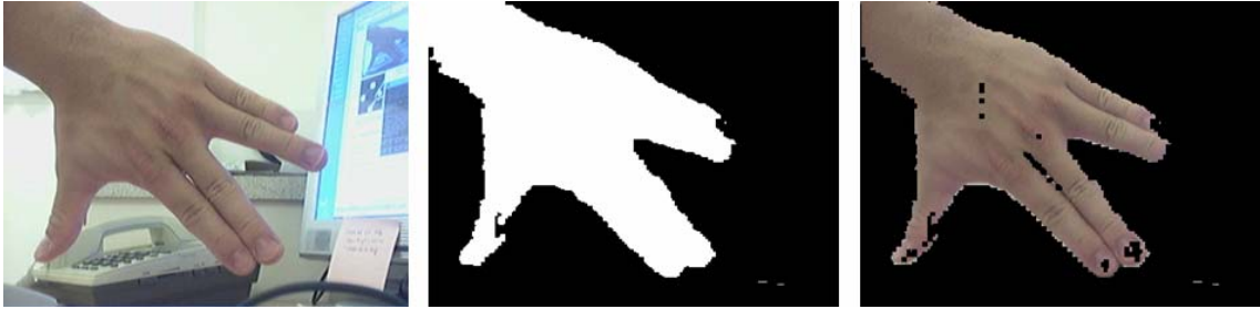
Figure 4. The image on left is colour-segmented to find the skin-colour pixels (middle image). The two images are then combined to produce the VideoArms image on the right.
