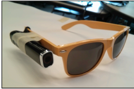
Figure 2: A Looxcie 2 camera attached to a pair of sunglasses.
