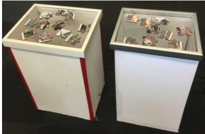
Figure 1: Puzzle Space consists of two paper boxes, transparent plastic frames, physical puzzle pieces and webcams.
