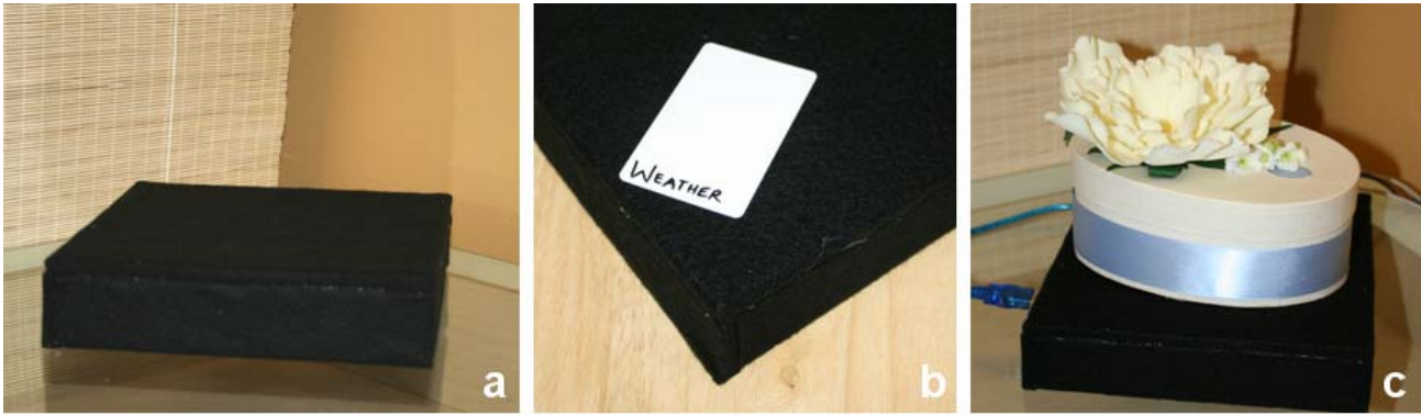
Figure 2 a) Smart location base. b) Information card assigns a data stream to a location. c) Appliance placed on a base.
