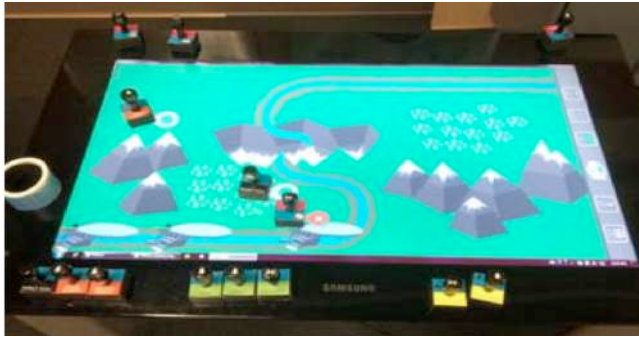
Figure 1. Youtopia: a collaborative hybrid tangible multi-touch tabletop sustainable land use planning activity.
