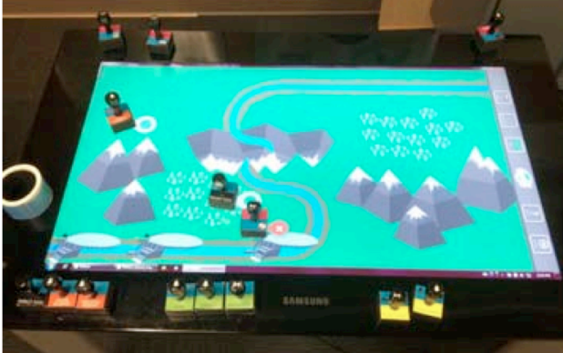
Figure 1. [Name removed]: a collaborative hybrid tangible multi-touch tabletop sustainable land use planning activity.
