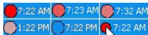
Figure 2: Virtual Intimate Object (VIO) in taskbar, showing color changes over a twelve hour period. Note initial rapid fading in top line. Final image shows display of remote partner’s button state on mouseover.
